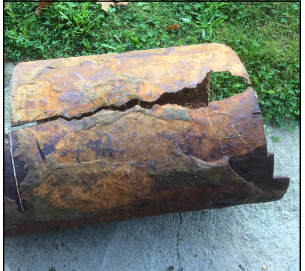
Above: The defective section of ductile iron pipe removed from the force main on the Bridle Path.
